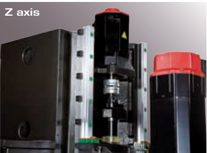
Z axial servo motor drives the whole weight of the spindle head
