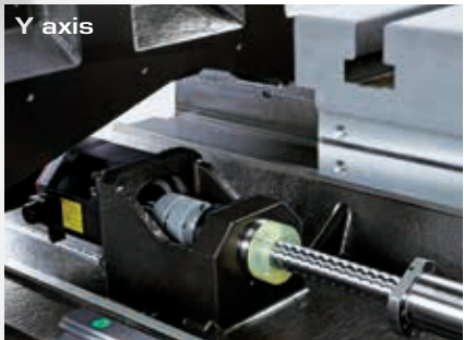
Casting in one piece for ball screw and bearing supports on all axes.
