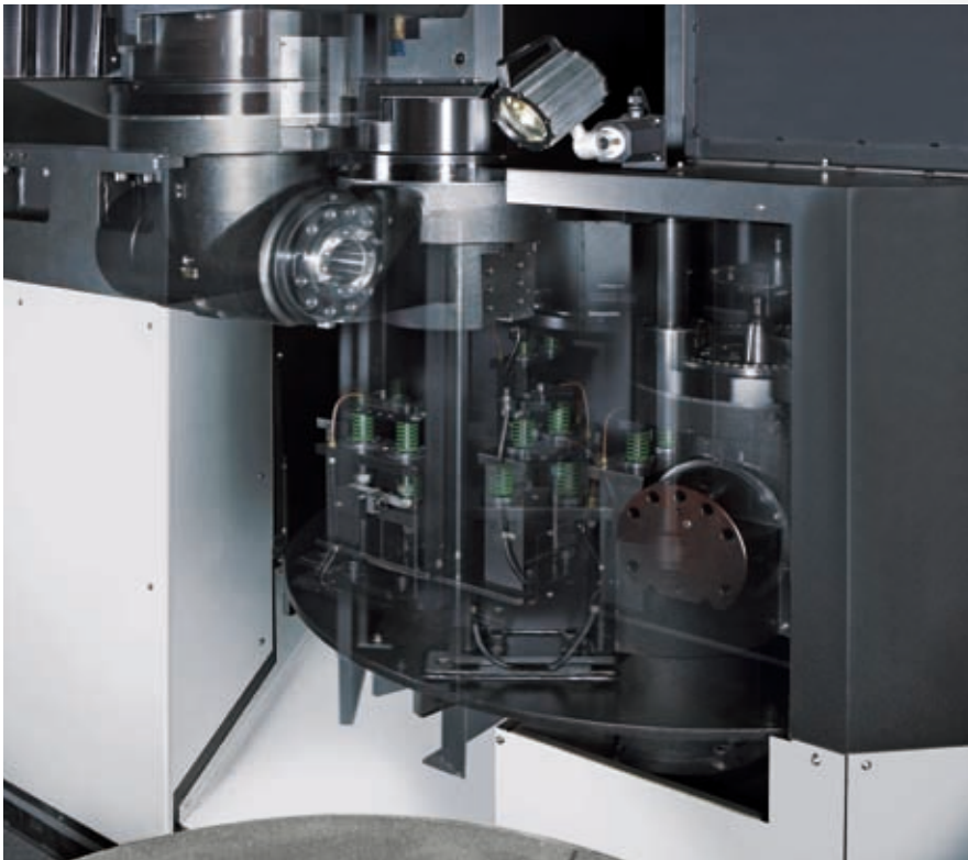
• Automatic head exchange system : Turning head, 90 degree head, and protect cover.
