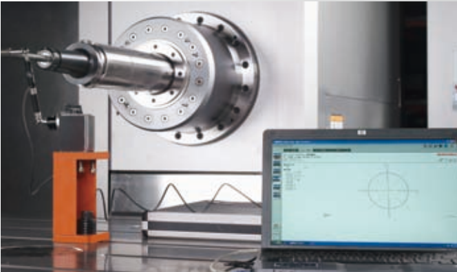
Ball bar Circular interpolation measurement.
