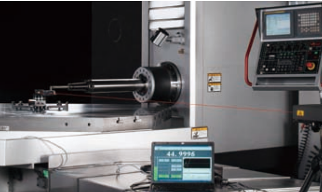
Positioning measurement (VD13441 standard.)
