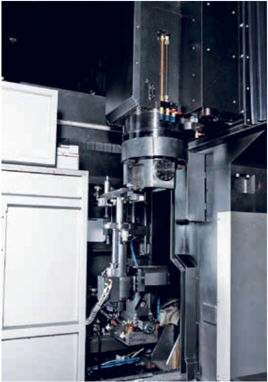
• Automatic tool exchange system in vertical/ horizontal/ turning tool.
