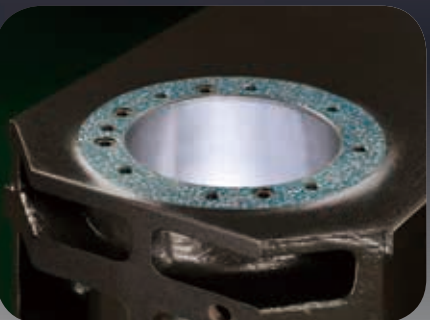
Every major contact surfaces are scrapped to ensure the geometric accuracy in top level and satisfy customers' quality demand.
