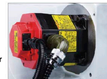
X.Y.Z-axis Driven by Servomotor
