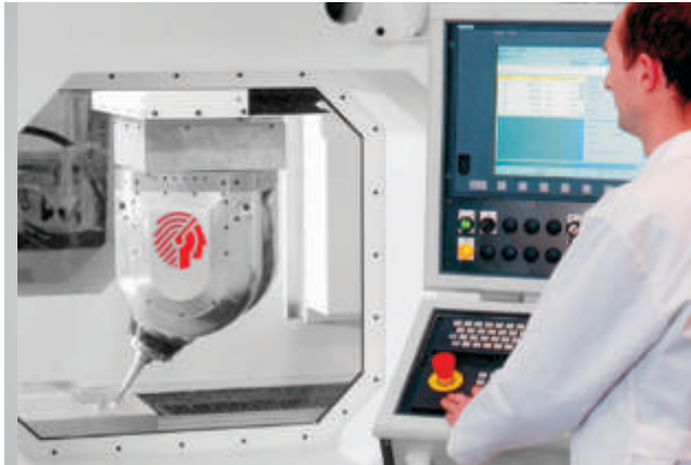
Structure integrating large glasses allowing an easy control of machining
