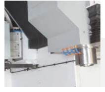
The Coolant nozzles around the Spindle face facilitates the manual adjustment of the nozzles for proper positioning of the coolant on the job while machining.
