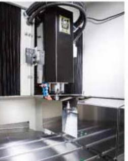
he Closed-Bridge type construction, combined with extra strong box type columns eliminate rigidity displacement while the spindle head is moving.
